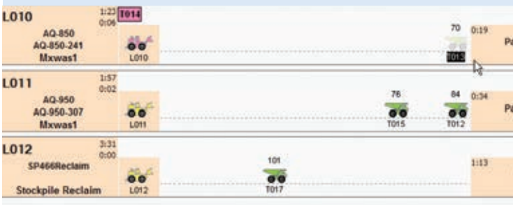
Fleet Control Dispatch Program – Manages truck assignments and load details for optimal production
